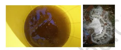
**Step 3** – Take out the tube and rub it with the AirOxi Cleaning Clamp (picture in previous page) to clean loose particles
